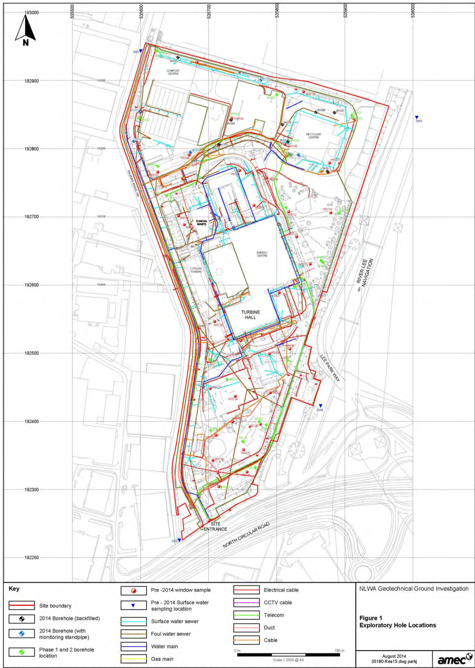
Figure 4 Borehole location plan
