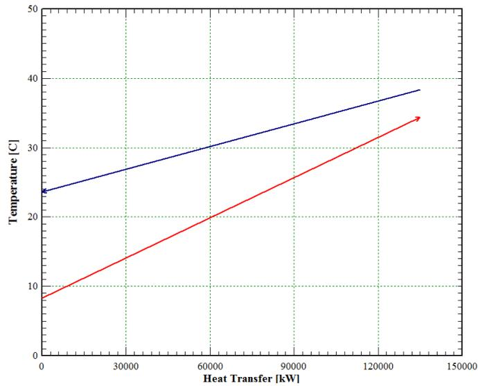
**Figure 17: Temperature (T) Heat transfer (Q) diagram for the cooling tower**
