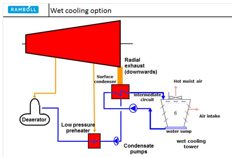
**Figure 12: Process setup of the cooling tower option**
