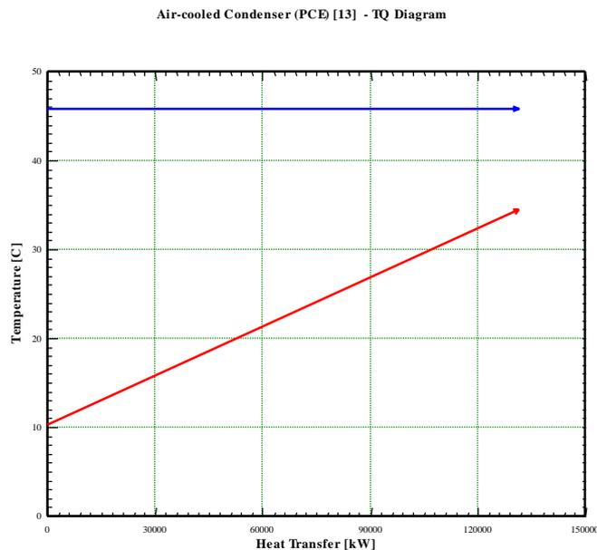
**Figure 7: Temperature and Heat (TQ) diagram for the ACC solution**
