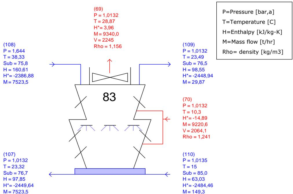
**Figure 20: Thermodynamic modelling results for the hybrid cooling tower option**
