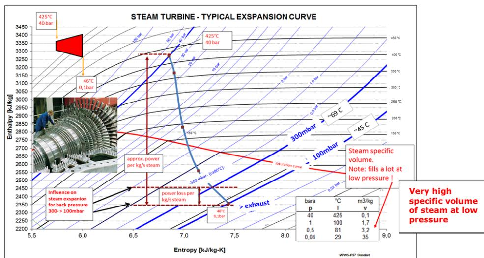
**Figure 2: Typical steam expansion curve (425 °C example)**
