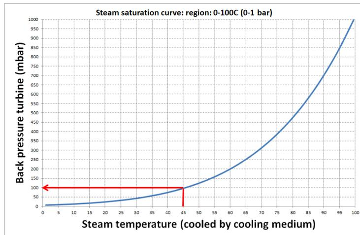
**Figure 1: Relationship between saturation pressure and temperature**
