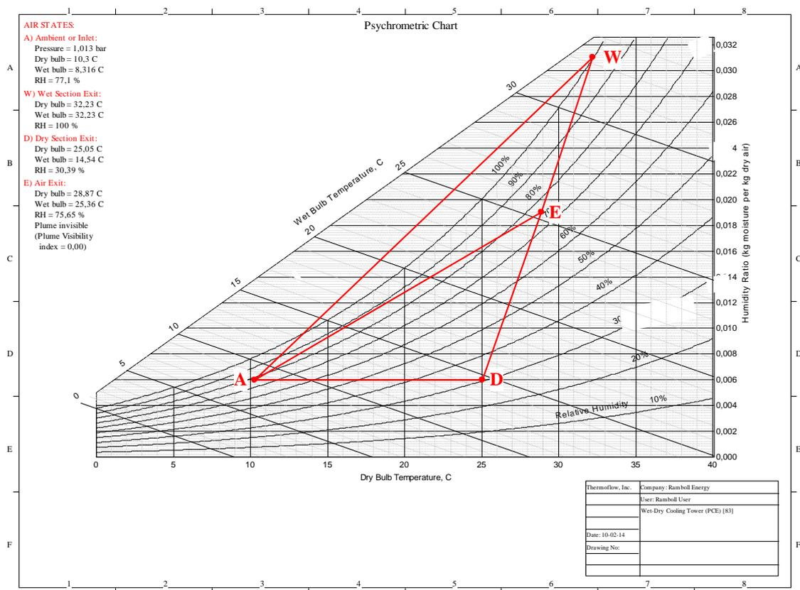
**Figure 21: Psychrometric chart for the air flow in the hybrid cooling tower at 10.3 °C ambient temperature**
