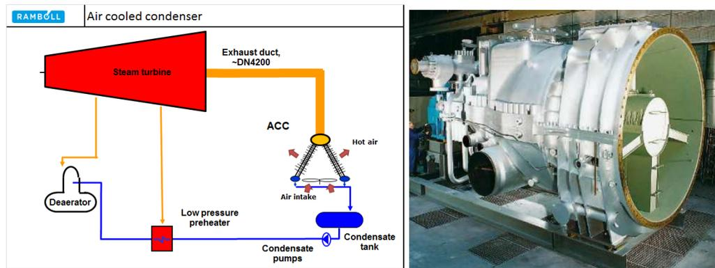
**Figure 4: Process setup for air cooled condenser (left). Turbine with axial exhaust (right)**
