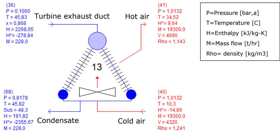
**Figure 6: Modelling results for the ACC system**
