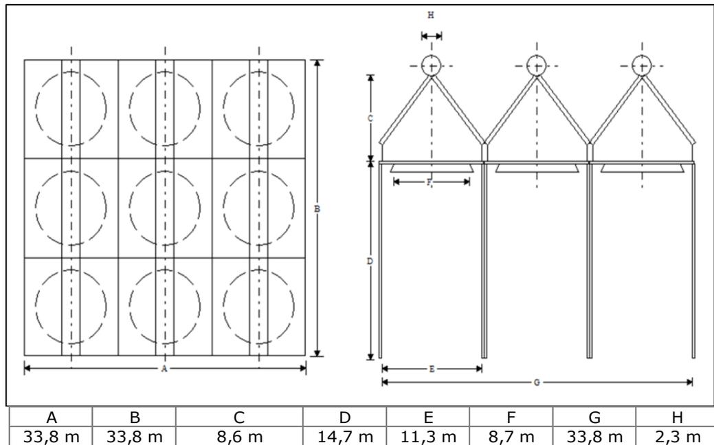
**Figure 8: Estimated physical layout of air cooling condensers**
