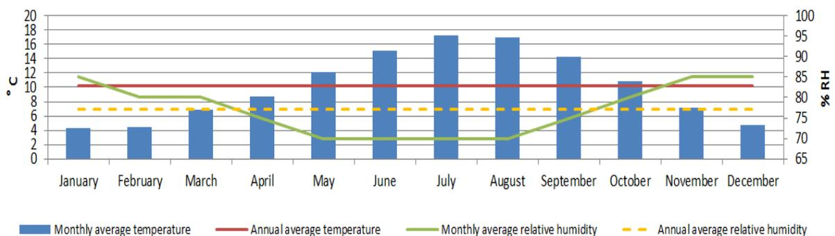
**Figure 3: Average temperature and relative humidity for London, based on 30 years of data**
