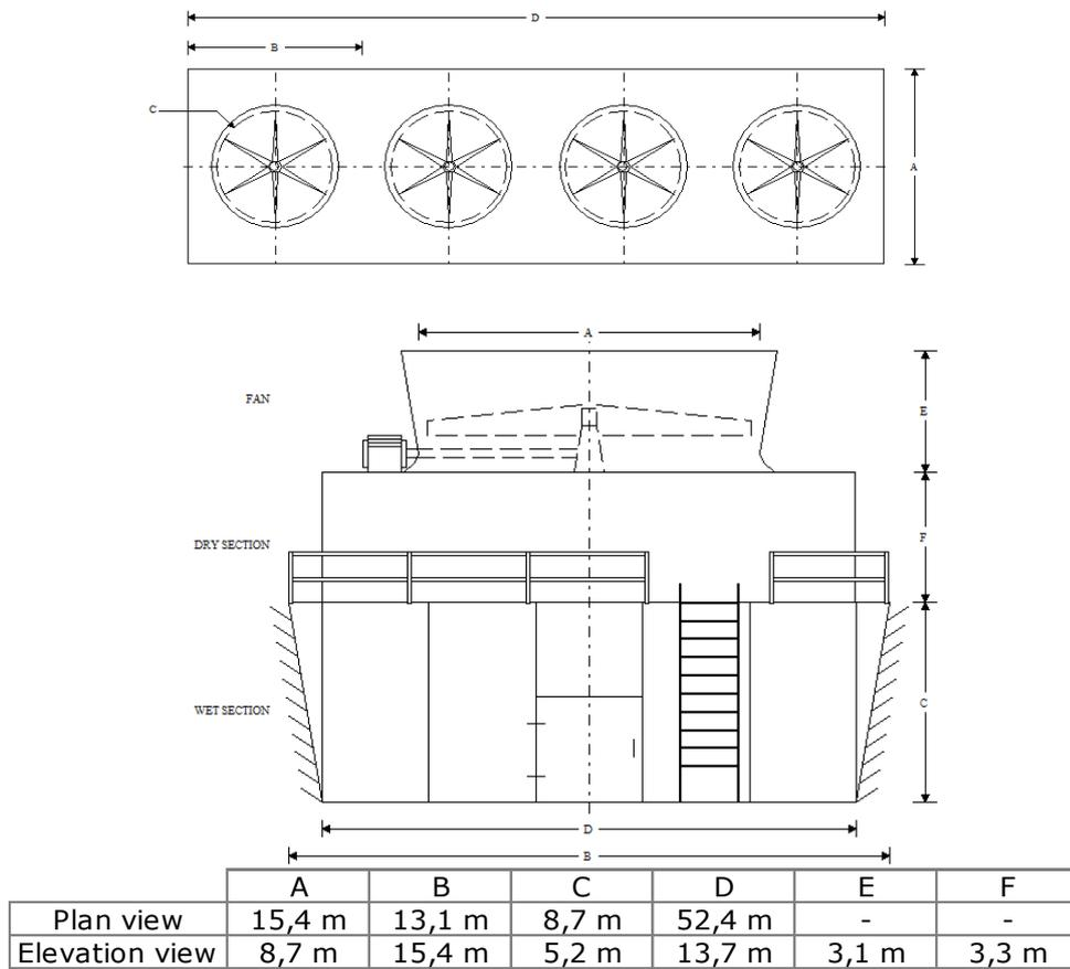
**Figure 23: Estimated wet cooling tower layout. Plan view (top) and elevation view (bottom)**
