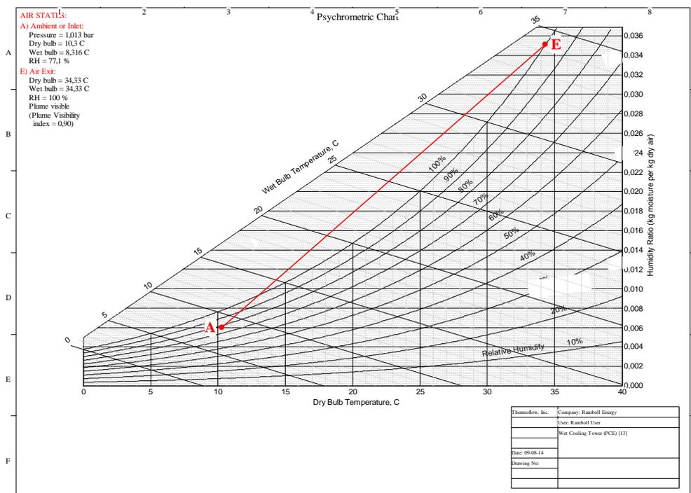
**Figure 18: Psychrometric chart for the air flowing into the cooling tower**
