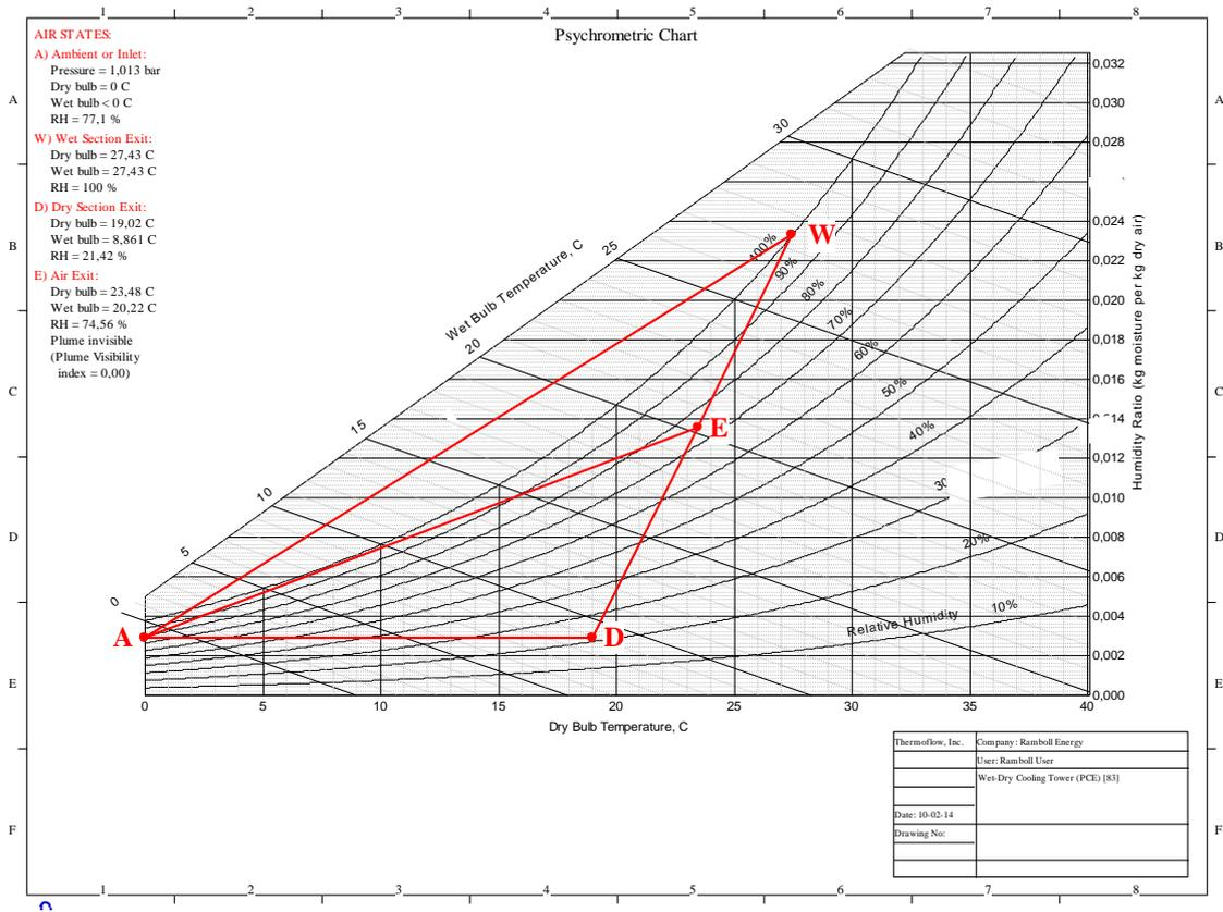
**Figure 22: Psychrometric chart for the air flow in the hybrid cooling tower at 0 °C ambient temperature**
