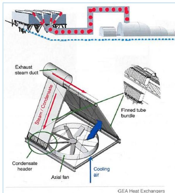
**Figure 5: Air Cooled Condenser unit, elevated to allow inflow of air from beneath**
