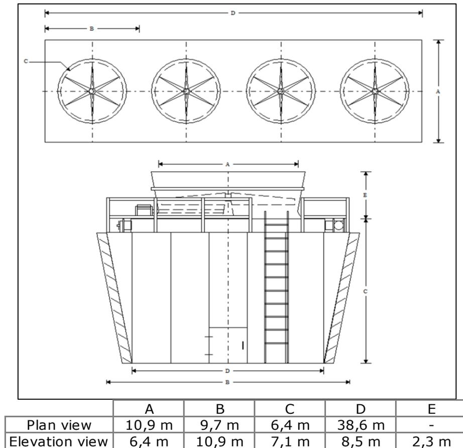
**Figure 19: Estimated wet cooling tower layout. Plan view (top) and elevation view (bottom)**
