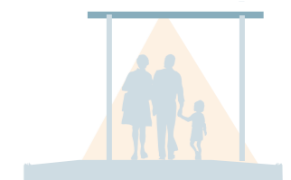
Down-lighting mounted to the underside of canopy
