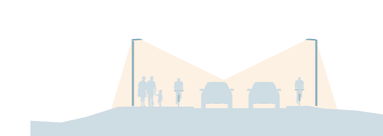
Narrow-ranged 3m high lighting for public routes to control light spillage
