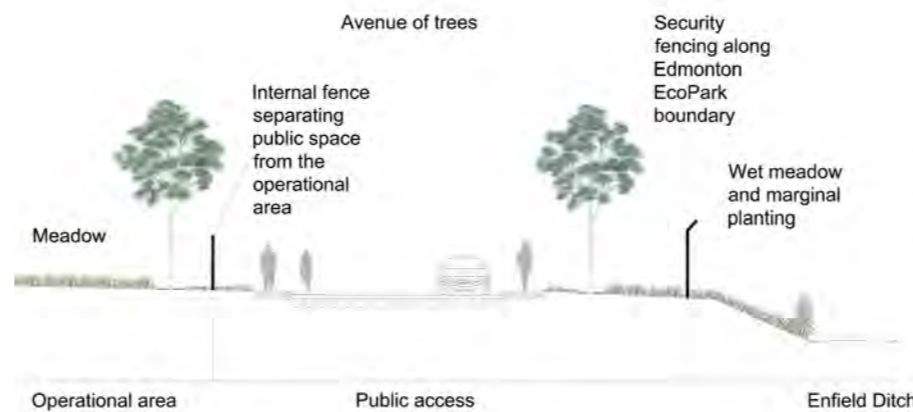
Figure 6.104: Illustrative section through internal access road
