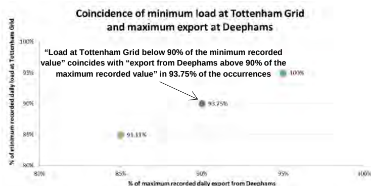
Figure 9 - Coincidence of minimum daily load at Tottenham Grid and maximum daily export at Deephams for the last three years
