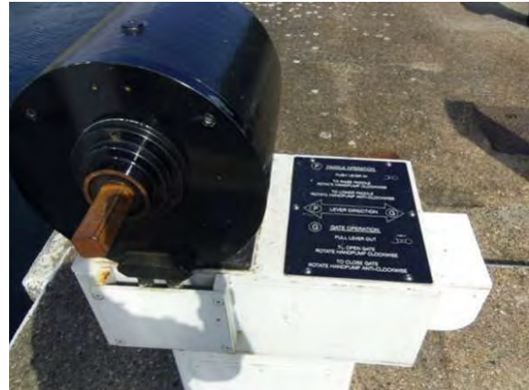
Figure 5-4: Hand-pumped hydraulic system
