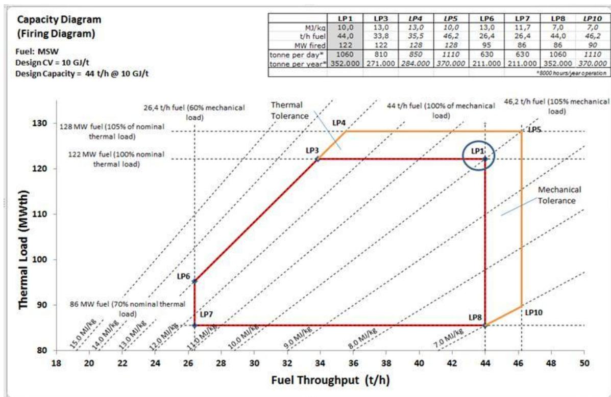
**Figure 2: Plant capacity diagram with a design CV of 10 MJ/kg (350 ktpa line)**
